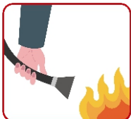
4 软管对准火源根部 Aim the nozzle at the root of the fire source
