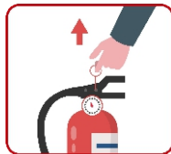
3 拔掉灭火器保险栓 Pull out fire extinguisher pin
